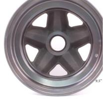
The Porsche 910, sometimes known as the Carrera 10, was originally raced in 1966 and 1967. It was based on the 906 series of Prototype Sports Cars and featued either a 2.0-litre flat-six or a 2.2-litre flat-eight. One of the distinctive features was its smaller 13" wheels, as per Formula One. The 9.5x13" rear wheel can be used on the front axle of the 908-3.
