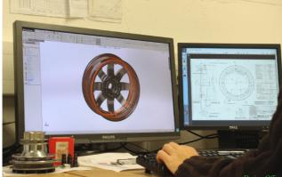
Every Crosthwaite & Gardiner part design is produced in-house by our dedicated design offices. Here, historic wheels and many other components are reverse engineered using both original components and original period drawings. The reproduction process includes the originals being measured and 3D modelled using our state of the art CMM (Coordinate Measuring Machine) and CAD (Computer Aided Design) software.
