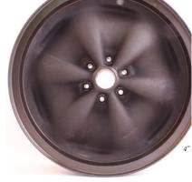
The instantly recognisable 'Wobbly Web' wheel first appeared on the 1957 Formula 2 Lotus Twelve; the design was formulated in order to achieve a lighter wheel, in typical Lotus fashion. A constant material thickness is used, with the tighter waves near the centre resulting in the greatest strength where it is most needed.
