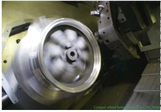
These castings are then finished in our machine shop, which features three CNC (Computer Numerical Control) lathes. Once machined and drilled where appropriate, magnesium wheels are cromated black for corrosion resistance. Some wheel models are also crack-detected and impregnated for deflation resistance. Please note that all of our wheels, with the exception of some Bugatti models, feature a safety bead allowing the safe use of tubeless tyres.
