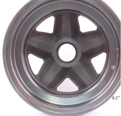
The Porsche 910, sometimes known as the Carrera 10, was originally raced in 1966 and 1967. It was based on the 906 series of Prototype Sports Cars and featured either a 2.0-litre flat-six or a 2.2-litre flat-eight. One of the distinctive features was its smaller 13" wheels, as per Formula One. The 9.5x13" rear wheel can be used on the front axle of the 908-3.
