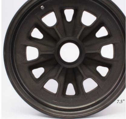
From its humble British Bristol-engined beginnings to the monstrous Ford V8-powered renditions, the Cobra remains one of the best recognised and iconic sports cars to enter racing history. This 'wine glass' wheel design was used in period and thanks to a 7.5" width, a greater range of fitments is available to cater for various types of bodywork and race series regulations.
